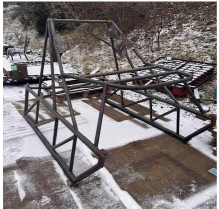
Figure 19: The new NIFCA camera frame designed to align with ICES WGNeps member institute specifications.
