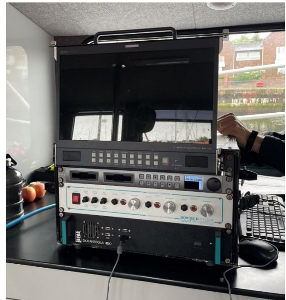
Figure 2 | Survey equipment set-up. Sledge camera unit (top left), comprising a Bowtech Surveyor-HD camera with three LED lights and two Z-bolt green point dive lasers (top right), contacted to the A-frame onboard St. Aidan (bottom left), and indoor monitor set up for camera analysis of live footage (bottom right).
