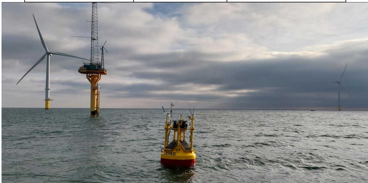
IWES Wind-Lidar-Buoy as deployed next to NOAH platform, off the coast of Blyth.
