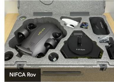
NIFCA has also made upgrades to our existing remote-operated vehicle (ROV) in the form of a FiFISH V6 Expert device that will further strengthen our existing survey capabilities.
