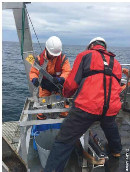
Grab samples carried out on Northumberland IFCA vessel St Aidan using a Van Veen grab in mud habitat to test indicators, including species diversity and total organic carbon.
